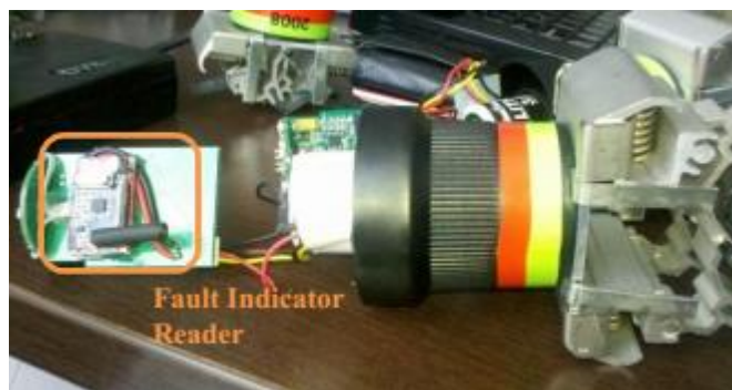
(a) Fault Indicator Reader (LFI for its acronym in Spanish) installed in the fault indicator. It is responsible to transmit the status of the equipment to the Fault Indicator Modem Reader through radio frequency. PIXIS Consultoría (www.pixis.com.co).
