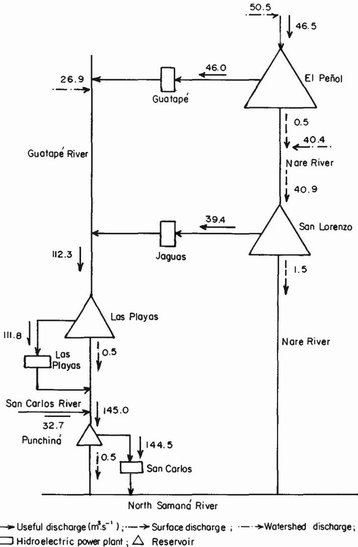
**Figure 1.** Part of the Nare-Guatapé hydroelectric system in Colombia, including the four reservoirs studied.
