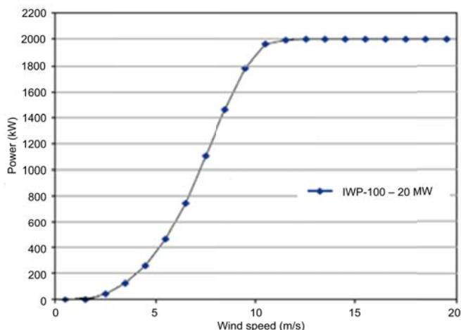
Fig. 4. Power curve vs. wind speed for a commercial generator FPC type of 2MW.
