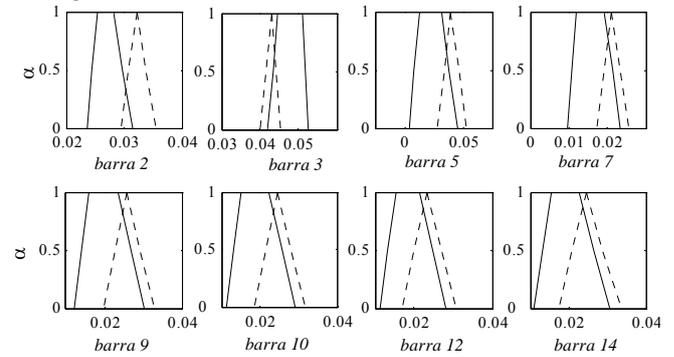
Fig. 7. Per unit 5th order harmonic voltage magnitude at buses 2, 3, 5, 7, 9, 10, 12 and 14. Dotted lines indicate the Possibility functions obtained in [12]; i.e. case *i*. Continuous lines indicate the Possibility functions obtained in case *ii*, i.e., by considering the wind farm at bus 2, and assessing the influence of the variability of the wind speed between the interval [5 mps – 20 mps].
