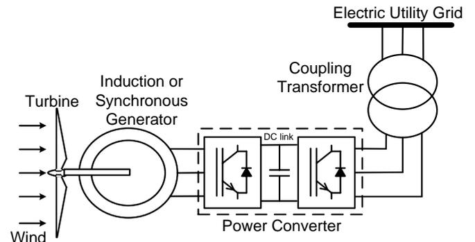
Fig. 2. Configuration of a FPC type wind turbine
