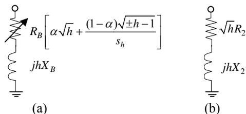
Fig. 3. Models to harmonic frequency for: (a) induction generators, (b) synchronous generators.
