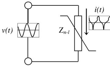
Fig. 1 Current harmonic distortion due to a nonlinear load
