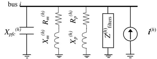
Fig. 5. General model of the aggregated load at a node of the PS
