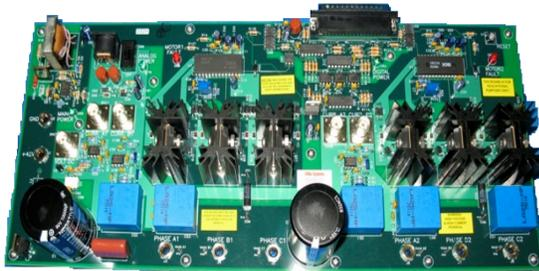
Fig. 2 Three Phase Power Inverter Board.
