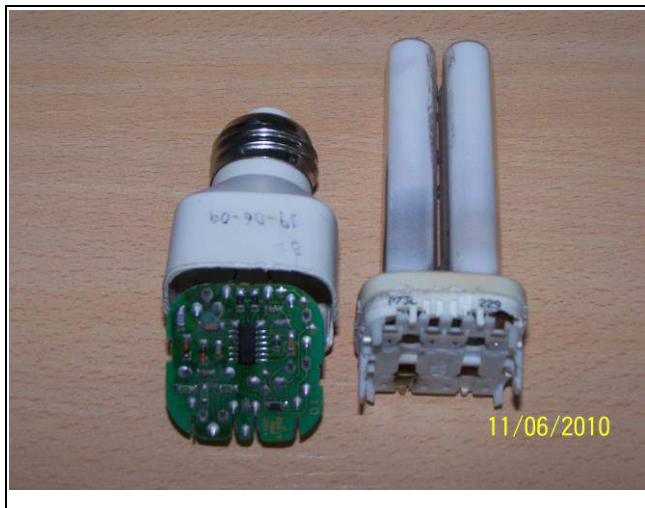
Figure 1. CFL functional parts. On the left, the electronic ballast and on the right the compact fluorescent lamp. (Lux America 2010).
