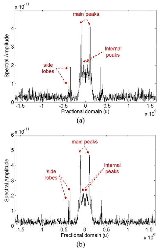
**Figure 6.** FRFT of the PD signatures. (a) Transform of signature PD008; (b) Transform of signature PD019
