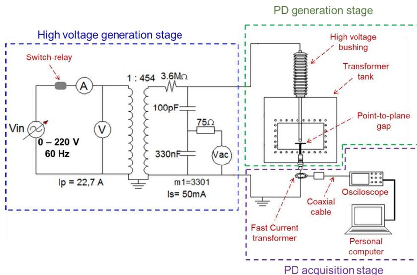
**Figure 3.** Experimental circuit used during the PD measurements
