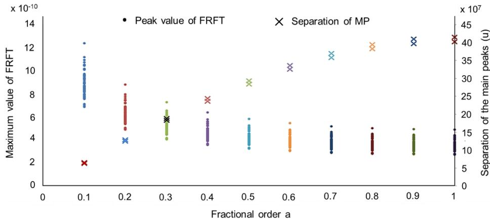
**Figure 7.** Peak value of the FRFT and separation between main peaks (MP) with respect to the fractional order  $a$
