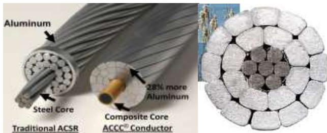
Fig.2: ACSR and ACCC conductor, Source: CEMIG, 2010
