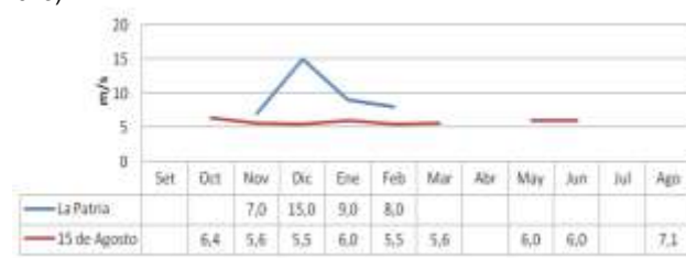
Fig. 5: Comparison of monthly average wind speeds in La Patria and 15 de Agosto . Source: Baez, 2011 and Mitjans, 2013.
