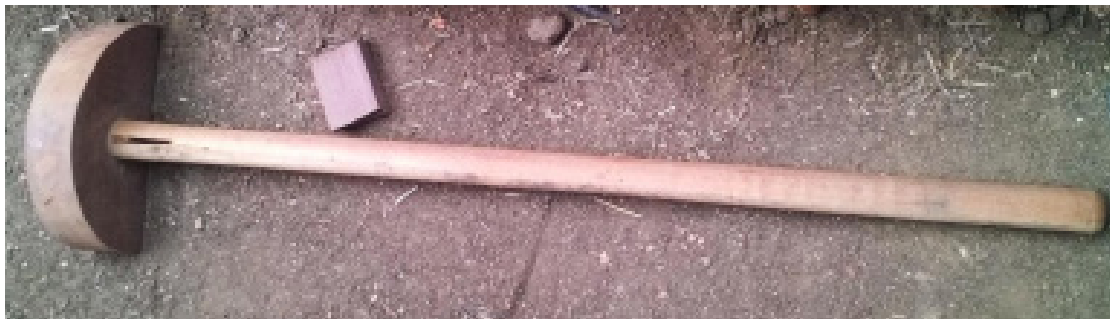
Figure 7. Puncher for soil compaction. Design: research team (Author, 2015).
