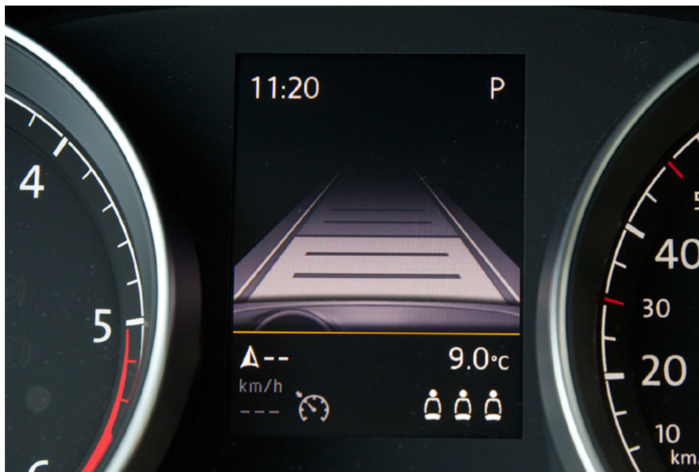
Figure 1. Adaptive Cruise Control is a driver aid which keeps the vehicle at a set distance from the one in front. Source: Nozilla. (2013). Adaptive Cruise Control vw Golf [Photograph]. Wikimedia Commons. https://commons.wikimedia.org/w/index.php?curid=25059896
