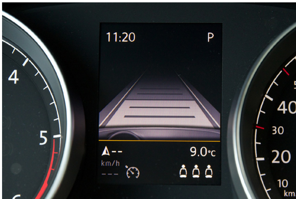
Figure 1. Adaptive Cruise Control is a driver aid which keeps the vehicle at a set distance from the one in front.
