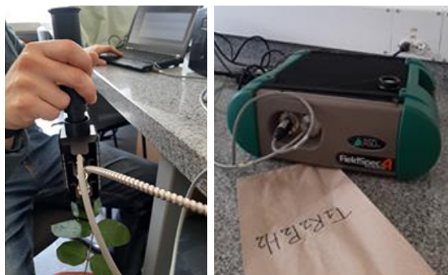
FIGURE 1. Capturing spectral responses: A) Leaf clip accessory, B) FieldSpec 4® spectroradiometer.
