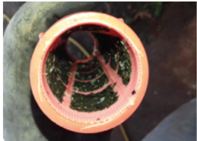
FIGURE 2. Screen filter clogged with particles from vinasse.
