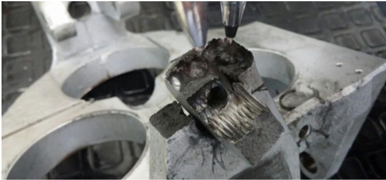
Fig 3. Image of the bubble in the piece of the surgical table.
