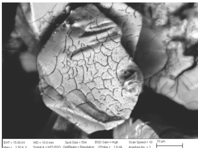
Figure 8. SEM image from the leaching residue of the -53+38\ \mu\text{m} particle size concentrate pre-treated with 15% of HCl.
