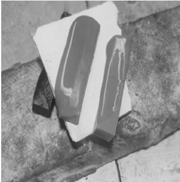
Figure 6. samples without coating, before annealing 200C, PLA material at 40% infill
