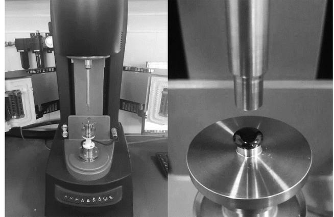
Figure 3. Dynamic shear rheometer (left), 8 mm geometry with the sample (right)
