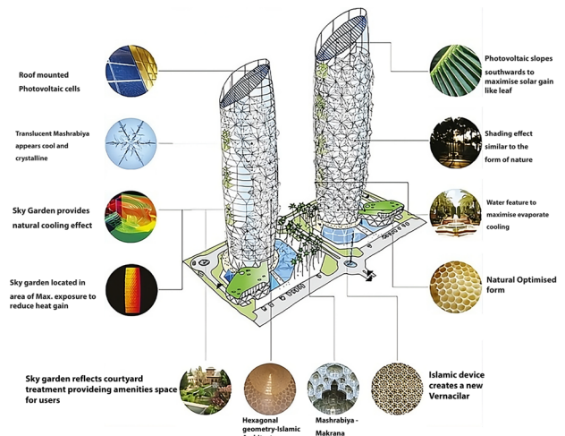
Figure 4: Demonstrates a dynamic Mashrabiya - inspired by the past is an adaptive natural system -Bahrain Towers in Abu Dhabi.
