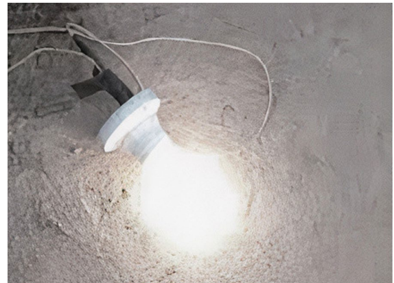
Figure 12. Shows exposing a room sample to lamp heat Source: Authers .2024
