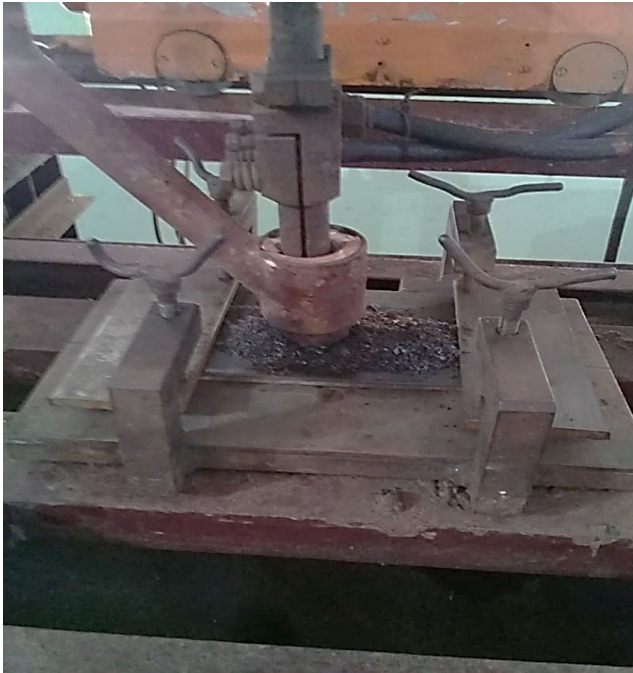
Figure 2. Deposition on fixed plate to achieve heat extraction and prevent deformation Source: Own elaboration
