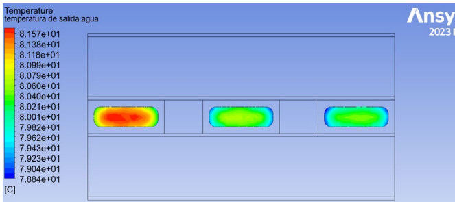
Figure 11. Temperature mapping at various water cooling flow outlets. Source: Own elaboration using Ansys Fluent®.
