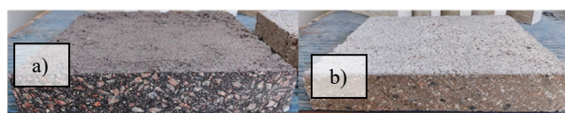
Figure 2. Cross-sectional cut in a) the reference specimen and b) the \text{TiO}_2 -modified specimen exposed to outdoor conditions for 12 months. Source: Authors' own work.
