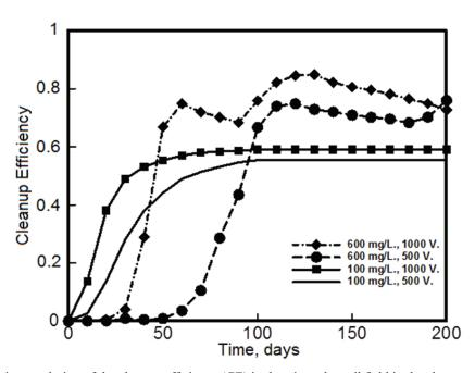
Figure 2. Predicted time evolution of the cleanup efficiency (CE) in the triangular soil field in the absence of wash water injection
