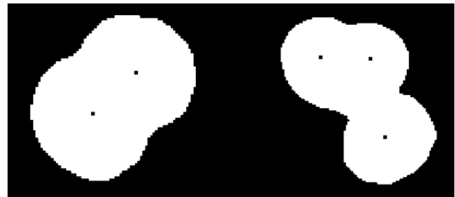
Figure 7. Centers detected by Hough in groups of two and three cells. Source: The authors.
