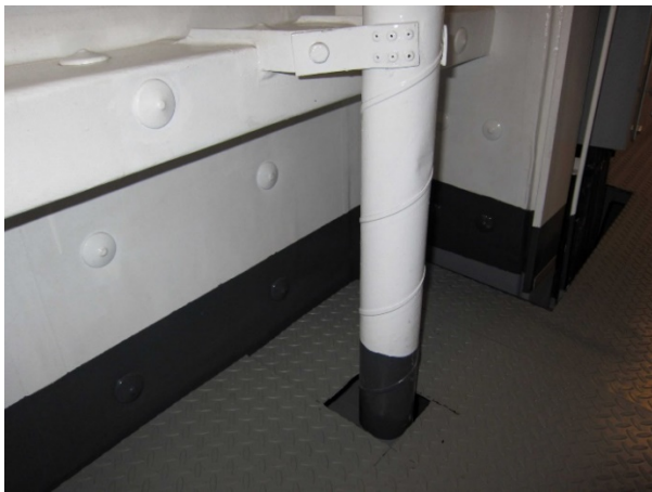
Figure 3. Lined bulkhead. Source: The authors
