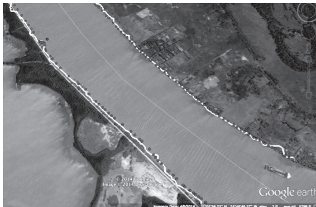
Figure 9. Comparison of the shore coordinates between the radar-based system and the data from IDEHA using a georeferenced image. Source: the authors.
