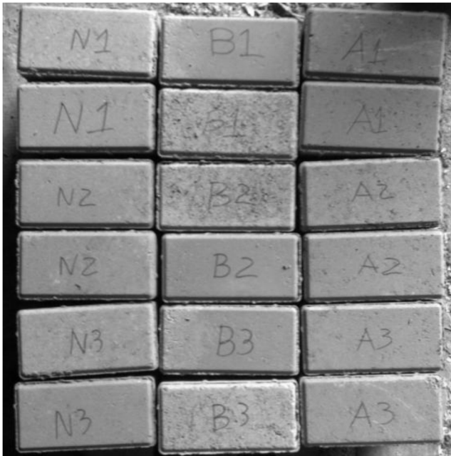
Figure 4. Concrete Paver Blocks for Visual Inspection and Laboratory Testing. Source: The authors.
