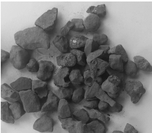
Figure 1. (a) BOF slag (b) BFD Source: The authors.
