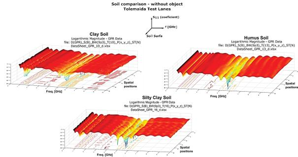
Figure 5. Image 1 shows images of three soils (Clay, Humus, and Silty clay) of the Tolemaida test lanes built with signals collected with a stepped-frequency GPR. These images show slight differences between 4 and 7 GHz. Source: The Authors.
