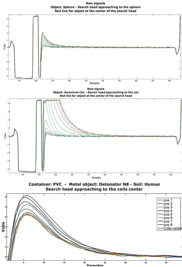
Figure 6. Metal Detector Prototype. Objects: Sphere, Aluminum Can, and Home-made landmine with detonator (Up to down). Las señales están dentro de medio periodo (periodo: 1 kHz, and 71 [sg/sample])
