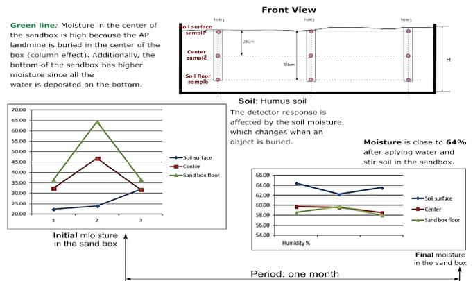
Figure 1. Front view of the sand box with humus soil, holes to collect soil samples, and soil moisture after to stir all soil content. A month before bringing the soil to the laboratory, it had a moisture level between 50% to 60%. This humus soil was brought from a village called Zipaquirá, two hours from Bogotá.
