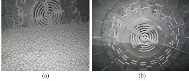
Figure 1: (a) picture of the mill before being unloaded; (b) picture of the mill after being unloaded. Source: The Authors.
