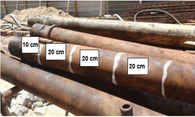
Figure 4. Marked sections on last meter of drilling rod.
