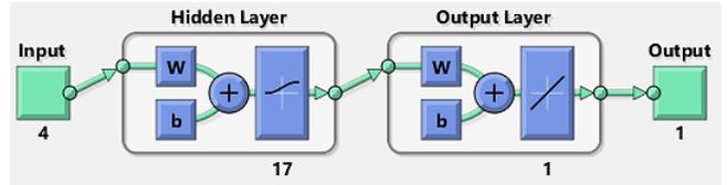
Figure 5. Structure of the NNA3 neural network. Source: own elaboration.
