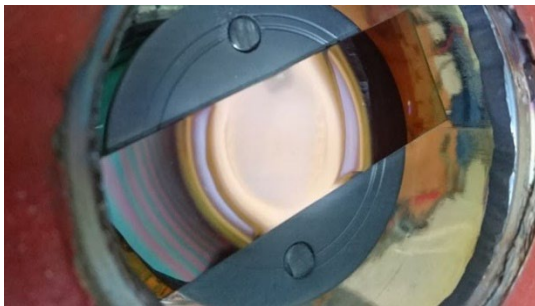
Figure 7. Copper coating on a glass substrate holder. Source: the authors
