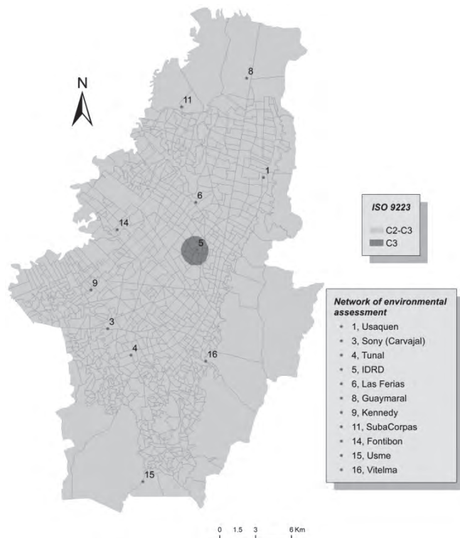
Figure 6. Map of atmospheric corrosion of carbon steel in Bogota, year 2011, according to ISO 9223 standard.
