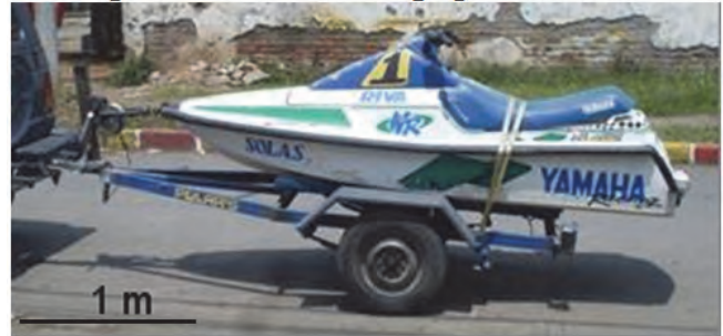
Figure 1. Strain gauge instrumented trailer Source: The authors
