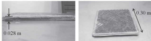
Figure 1. Panel of manufactured composite. Source: The authors.
