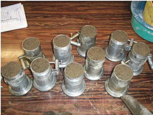
Figure 4. Cylindrical specimens of dimension 5 cm x 10 cm. Source: The authors
