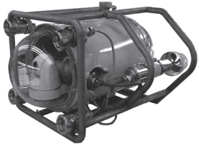
Figure 1. Underwater remotely operated vehicle Visor3. Source: [13]
