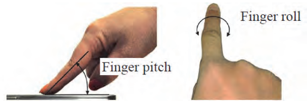
Figure 3. Illustration of the finger pitch and the finger roll. Source: The authors
