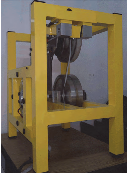
Figure 4. The ABS laboratory setup [11]. Source: Inteco Manual [11].
