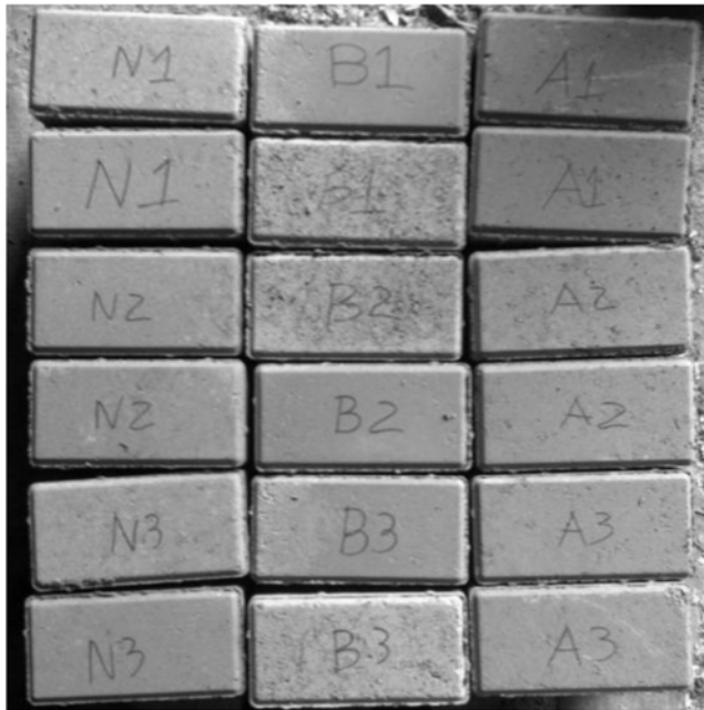
Figure 4. Concrete cover blocks for 8 visual inspection and laboratory tests. Source: The authors.
