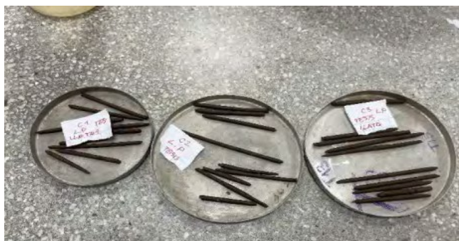
Figure 2. 3.2 mm thick bars to determine the PL of C-3 clay soil samples.
