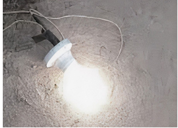
Figure 12. Shows exposing a room sample to lamp heat Source: Authors .2024
