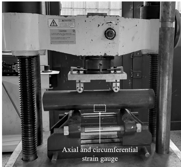
Figure 1. Four points bending-test Source: The author
