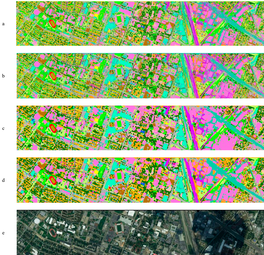
Figure 4. Classification maps for the Houston 2013 dataset: (a) SVM, (b) RF, (c) HybridSN CNN, (d) Modified HybridSN CNN, and (e) true color composition
