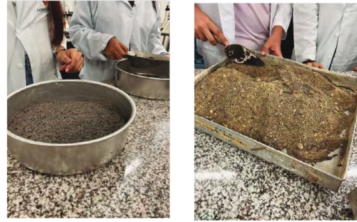
Figure 3. Mixture of Coal Ash with natural soil.
