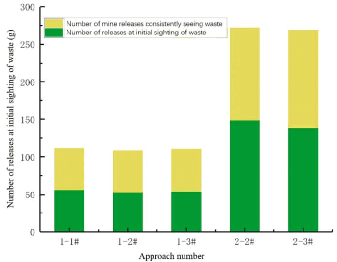
Figure 8. The relationship between different approaches and the number of ore release
