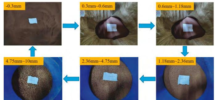
Figure 2. Ore of each particle size during the experiment
