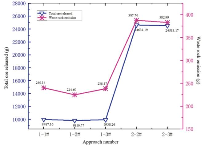
Figure 7. The relationship between different inlets and the total amount of waste rock released and the amount of waste rock released
