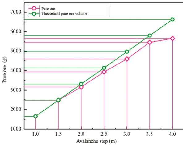
Figure 6. Relationship between different crumbling steps and pure ore volume and theoretical pure ore volume
