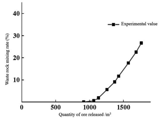
**Figure 11.** Relationship between ore release and waste rock mixing rate.3. Evaluation results
