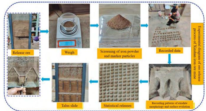
Figure 1. Flow chart of Xinshan iron ore release simulation experiment
