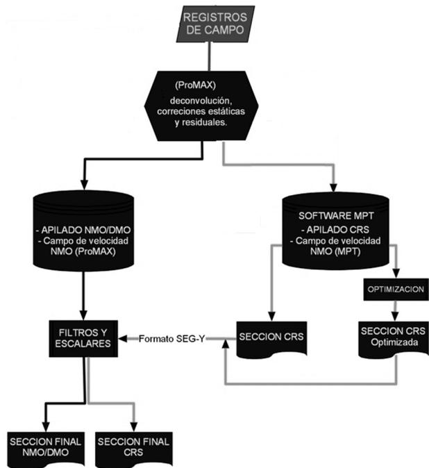
**Figure 2.** The CRS sequence differs from NMO sequence in velocity analysis and stacking steps where instead, searching and optimization of CRS parameters are used.
