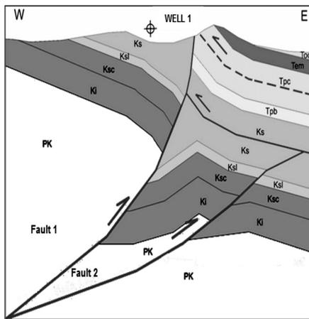
**Figure 4.** Geological section of the zone with several structural styles observed and a well at West, from an interpreted stacked section (internal report).
