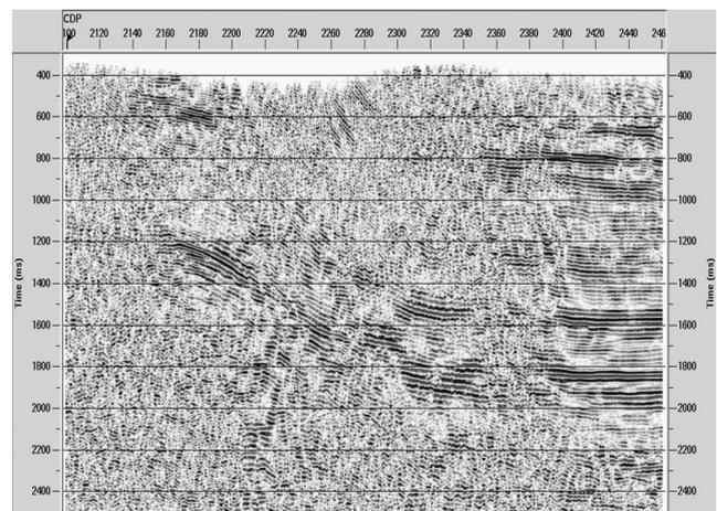
**Figure 6.** In the new NMO Stack section CDPs 2100-2460 the reflectors are observed along the whole section, including at left of CDP 2380.
