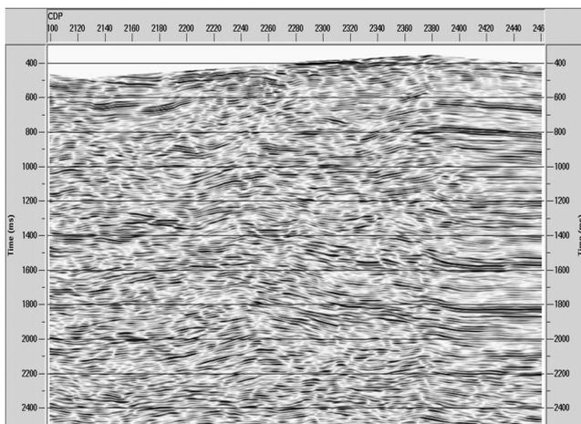
**Figure 5.** In the previous PSTM section CDPs 2100-2460, clear reflectors are observed from CDP 2380 to the right but blurred at left.
