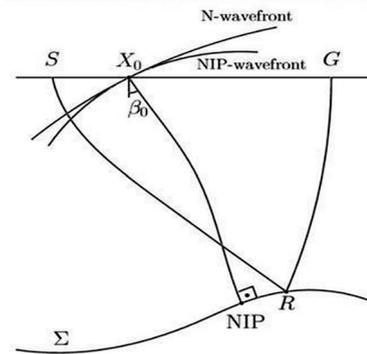
**Figure 1.** The Central ray is perpendicular to the reflector  $\Sigma$  and emerges at  $x_0$  with an  $\beta$  angle. The NIP and N waves reach the surface at point  $x_0$ .
