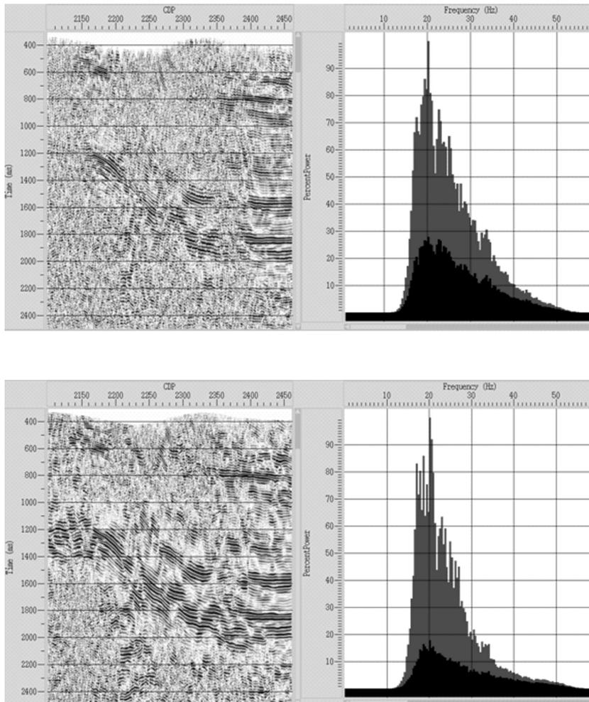
**Figure 8.** NMO at top and CRS at bottom images with respective spectral analysis show reduction in the level of random noise.
