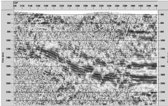
**Figure 7.** The CRS stack section CDPs 2100-2460 displays an enhanced image with better continued and more clear reflectors along the section.
