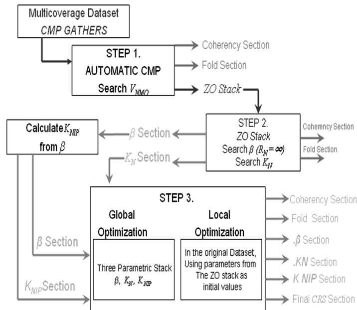
**Figure 3.** Flow charts with step sequence to obtain final CRS stack section.
