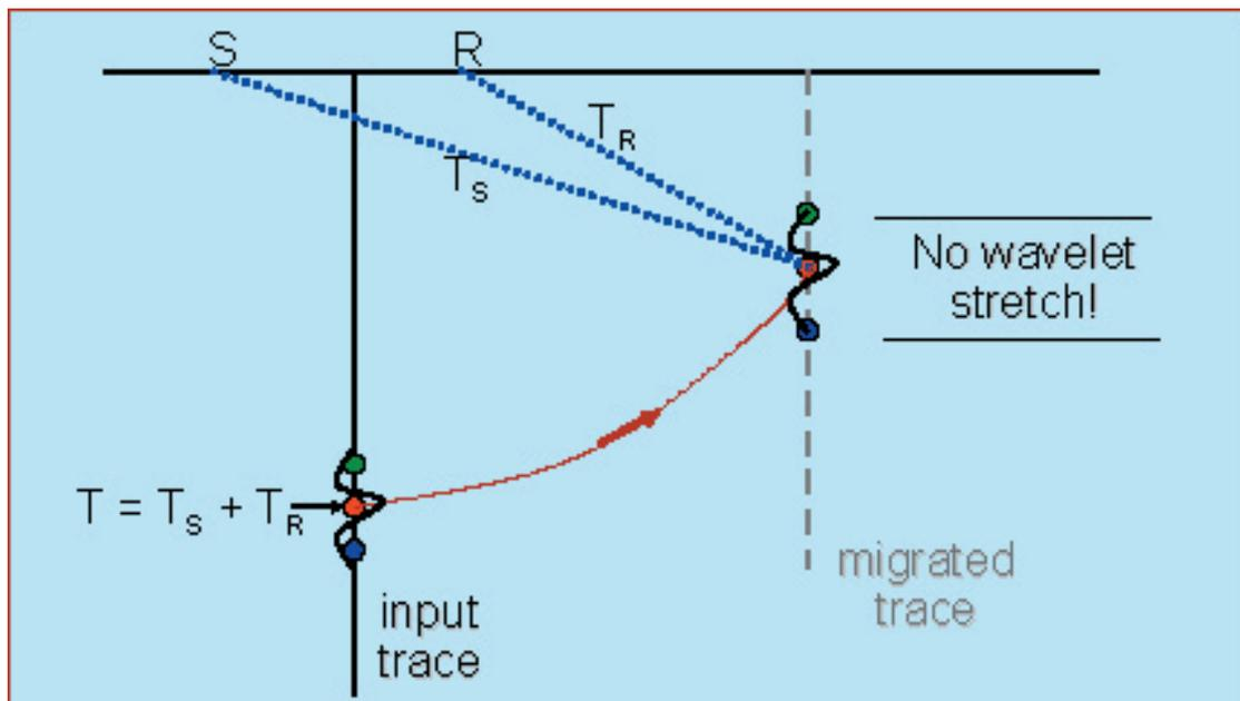
**Figure 2.** Instead of “moving” individual samples independently, a block of samples is moved along “parallel” paths so that relative separation between samples is not altered, hence no stretch is introduced. Ideally the block of samples should include the wavelet associated to the event of interest. This is a modification of the operation shown in Figure 1.
