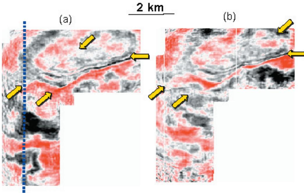
**Figure 6.** Comparison of time slices on the full offset range for the: (a) conventional and (b) target oriented migrations. Slice is taken at 1.2 seconds, approximately the time of the target horizon. Faults trending to the NE can be identified between the yellow arrows in each image.
