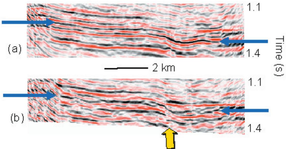
**Figure. 5.** Comparison between images from the conventional and the target oriented migration. Images stacked in the far-offset range. Once again the fault pointed-to by the yellow arrow is better resolved in the target-oriented image.
