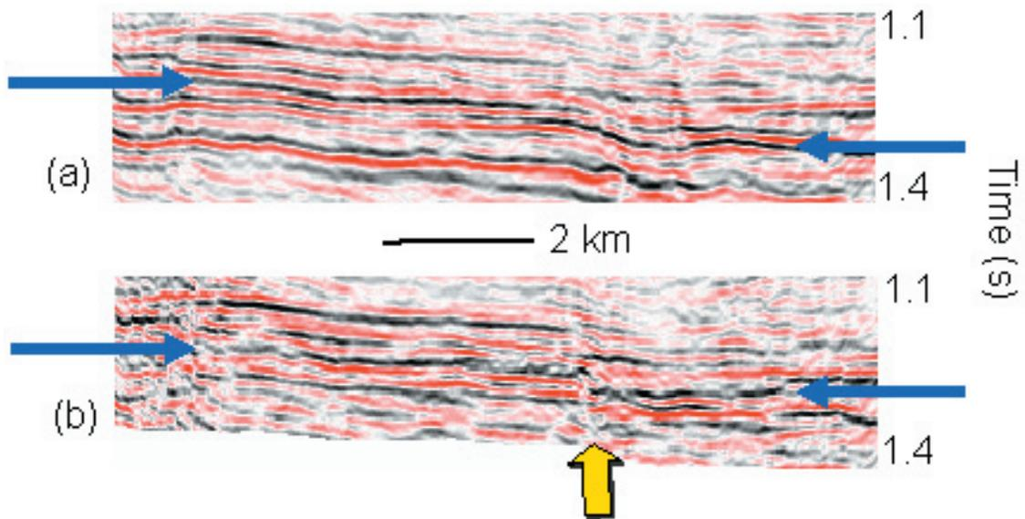
**Figure. 4.** Comparison between images for a selected inline from the 3D volume for the: (a) conventional and (b) target oriented migrations. Images stacked over the full range of offsets available to each migration. The blue arrows in each image point to the location of the event used as a target in the target-oriented migrations. The yellow arrow points to the location of a fault that is better resolved in (b).
