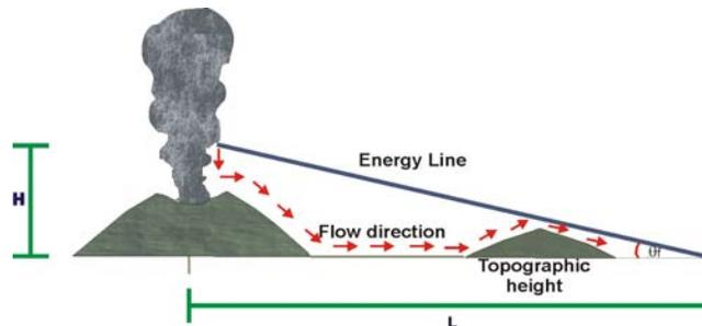
Figure 4. Energy line for Pyroclastic flows.
