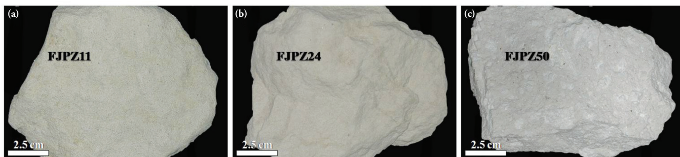
Figure 3. Hand-specimen photographs of the raw geomaterials. (a)-(b) Very fine- to fine-grained sandstones. (c) Volcanic tuff with the pumice lapilli clasts within the fine ash matrix.
