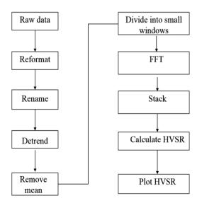
Figure 3. HVSR workflow chart of ambient noise processing in SAC and Geopsy software.
