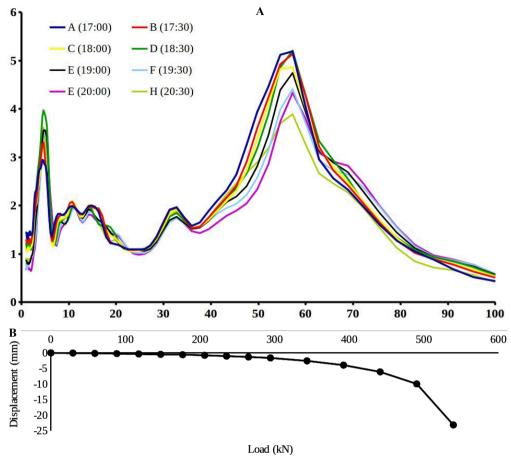
**Figure 4.** Results of the pile load test: (A) The HVSR curves obtained at each loading increment (30 minutes). Three peaks were observed: first (5Hz), second (32Hz), and third (55Hz), (B) The load-displacement curve of the pile compression load test.
