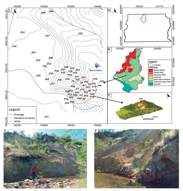
Figure 1. Location of Ribeirão Contagem watershed on Federal District map and its geology (A, B); Sobradinho landslide along the HVSR measuring points (red dots), red dashed ellipse is the approximate landslide boundary (C); Zoomed image of the landslide with a triangular array used for time-lapse monitoring (D); Photographs of the landslide (E, F).
