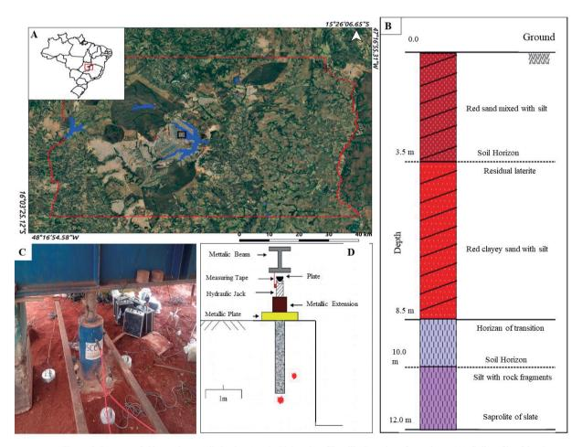
Figure 2. Prototype field experiment (pile load test) at the University of Brasilia. Location of experiment (A); Soil profile of the site (B); Photograph of the experiment (C) and Schematic of the loading mechanism (D).
