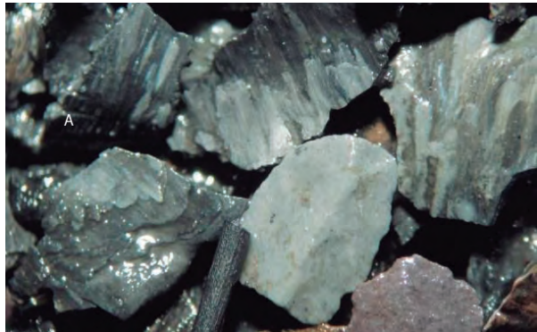
Figure 28. Mudstone medium grey. (A) metamorphosed cuttings. (B) unaltered chips from Los Cuervos Fm. Drilled with impregnated bit + turbine & OBM.
