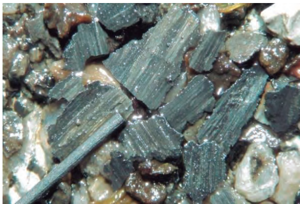
Figure 18. Sandstone medium dark grey with metallic lustre from Mirador Fm. Drilled with PDC bit & OBM
