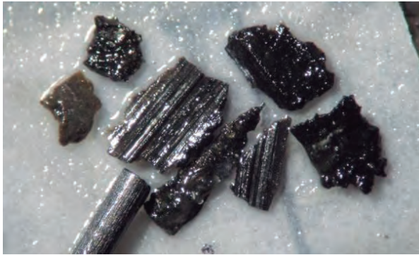
Figure 17. Sandstone greyish black with metallic lustre from Guadalupe Fm. Drilled with impregnated bit & OBM.
