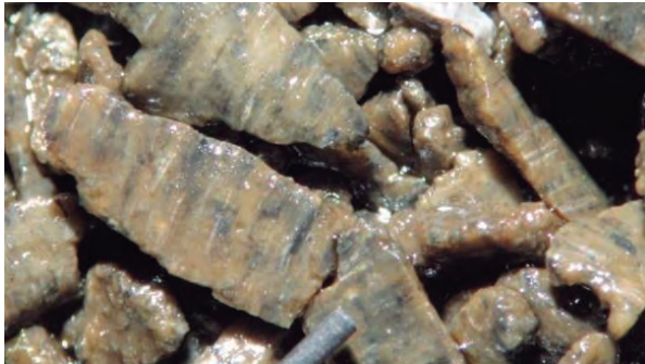
Figure 30. Sandstone pale yellowish brown with black & white streaks due to quartz & lithic grains from Mirador Fm. Drilled with tricone/PDC bit & OBM.
