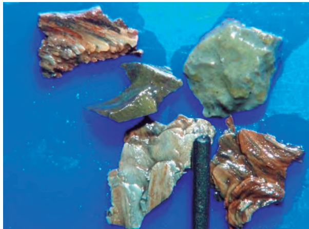
Figure 29. Mudstone medium grey with moderate red mottled, metamorphics & platy from Los Cuervos Fm. Drilled with impregnated bit + turbine & OBM.
