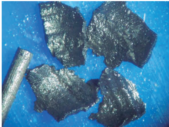
Figure 25. Mudstone dark grey, grooved flakes from Mirador Fm. Drilled with PDC bit & OBM.
