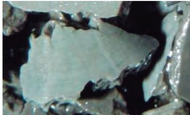
Figure 9. Mudstone greenish grey from Carbonera C8 Fm. Drilled with PDC bit & OBM.
