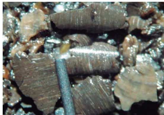
Figure 11. Siltstone yellowish brown & Sandstone greyish yellow from Mirador Fm. Drilled with PDC bit & OBM.
