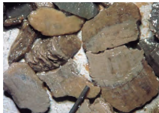
Figure 10. Mudstone moderate brown with laminations of Sandstone pale yellowish brown from Mirador Fm. Drilled with PDC bit & OBM.
