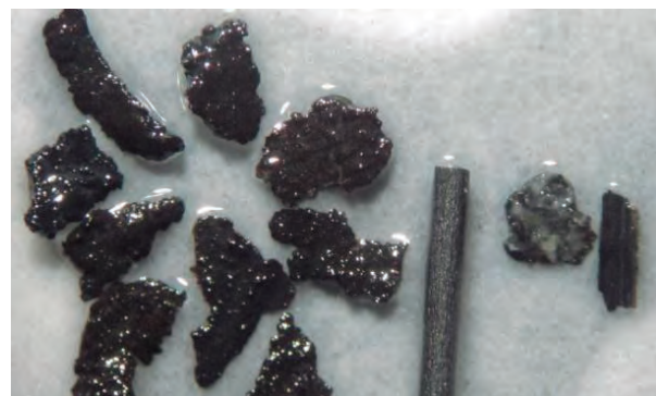
Figure 23. Sandstone black from Mirador Fm. Drilled with impregnated & OBM.
