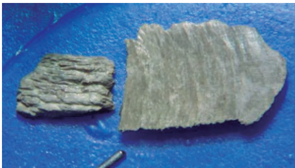
Figure 7. Mudstone medium grey from Guadalupe Fm. Drilled with PDC bit & WBM.
