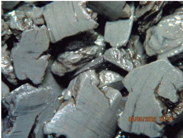
Figure 6. Mudstone medium grey from Carbonera C8 Fm. Drilled with PDC bit & OBM.
