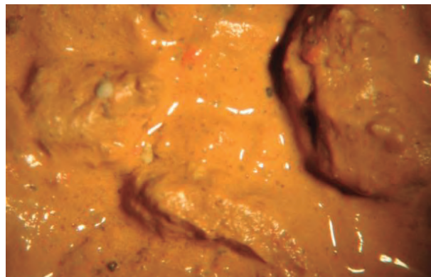
Figure 5. Mudstone reddish brown, moderate yellow, amorphous & blocky from Guayabo Fm. Drilled with PDC bit & WBM.
