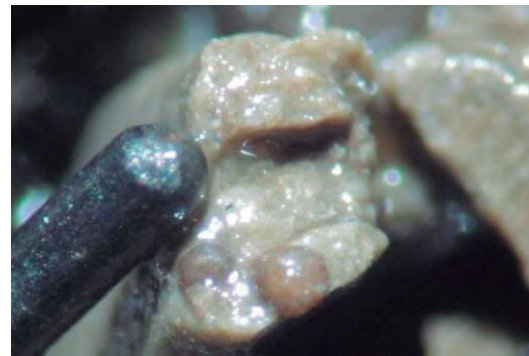
Figure 41. Mudstone light yellowish brown with siderite nodules (magnification x32) from Carbonera C7 Fm. Drilled with PDC bit & WBM.
