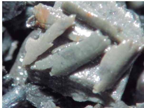
Figure 16. Siltstone light grey to white from Carbonera C8 Fm. Drilled with impregnated bit + turbine & OBM.
