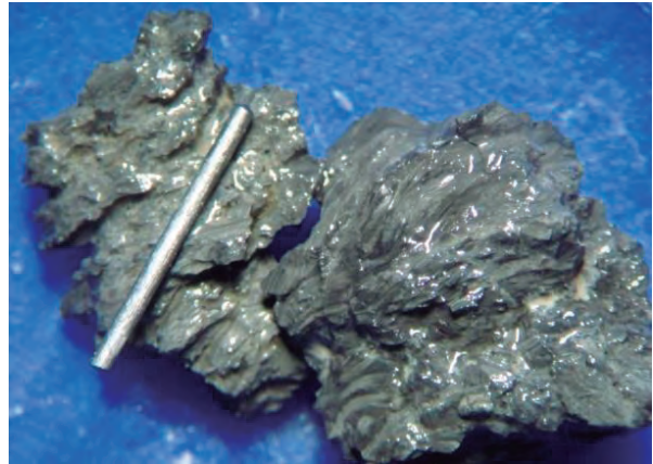
Figure 27. Mudstone dark grey, wrinkled, micro-banded lumps from Guadalupe Fm. Drilled with PDC bit & WBM.
