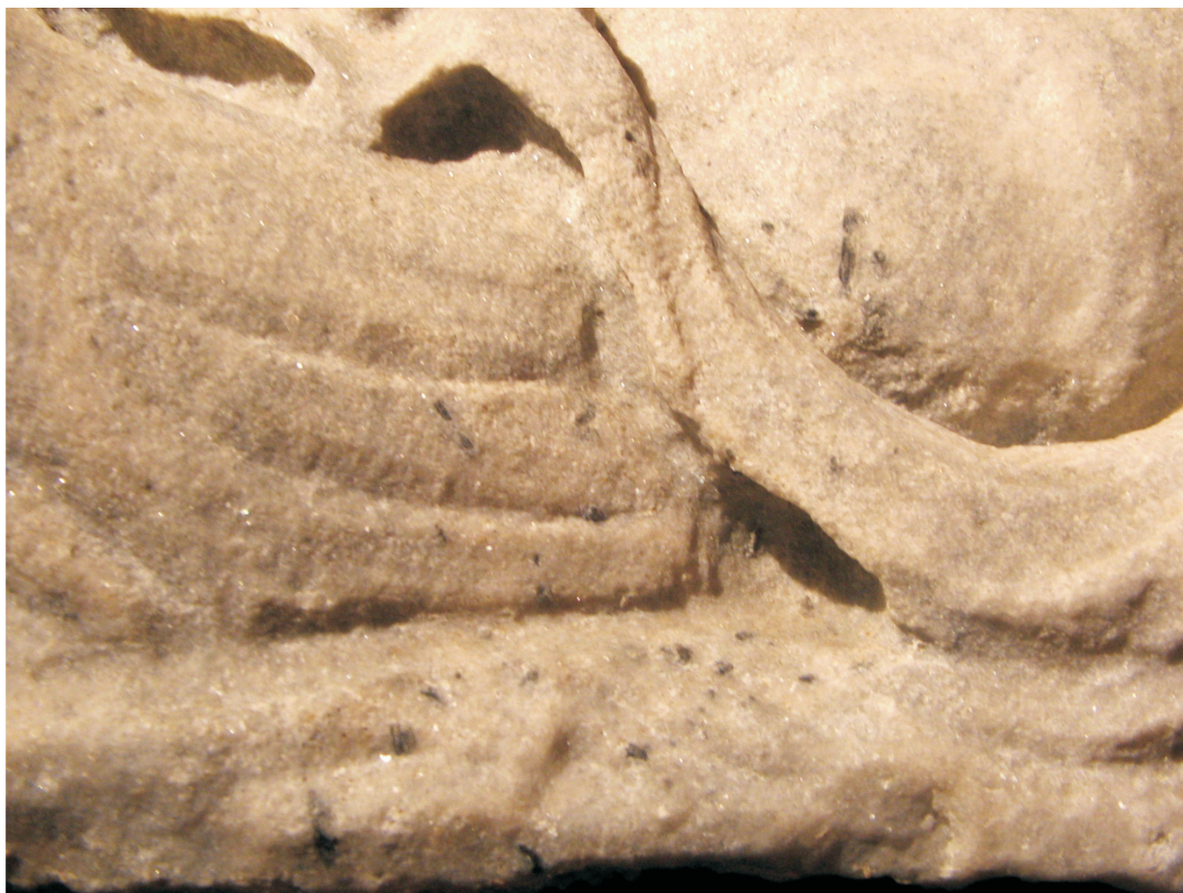
Figure 3: Platy hornblende and muscovite, characteristic of Hiesberg marble from the Großweichselbach quarry detail central part from Fig. 2; picture width: 21 cm.
