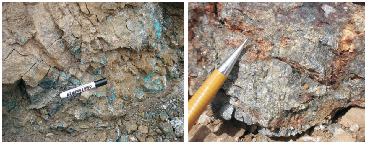
Figure 7: Right) Malachite mineralization in the fractured quartz diorite unit, Left) a close up of arsenopyrite mineralization together with quartz and Fe-oxides in fractures
